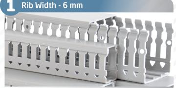
Since the rib width of the wiring ducts is designed as 6 mm, it will be sufficient to break only one rib for leading multiple or thicker cables through rib clearances. Thus, you will prevent cables hanging in the ribs as no multiple tabs are broken.
