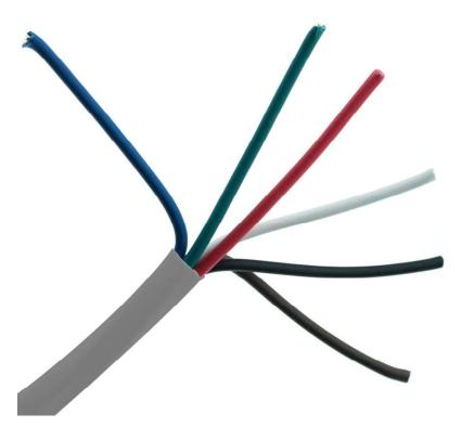
Cable Description: 6 Core alarm cable Conductor: 6C\*7/0.2mm Pure Copper (24AWG OFC) Insulation: PVC Insulation Thickness (mm): 0.25mm Insulation Dia. (mm): 1.0±0.08 Insulation Color: Red; white; green; red; Blue; Yellow; Black Nylon rips cord: 150D Jacket: PVC White Thickness : 0.6mm Overall Dia. (mm): 4.6mm±0.2 Packing 100m/roll, 200m/roll, 300m/ roll
